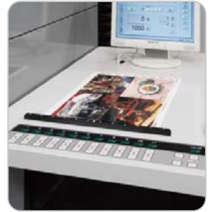
The ink keys are automatically preset on the DirectPress DI.
