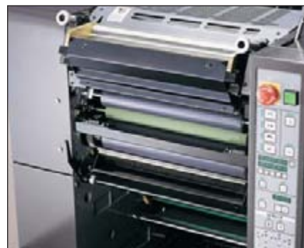
The ink system provides superior screen quality as well as the ability to print large, dense solids over the maximum printing area.
