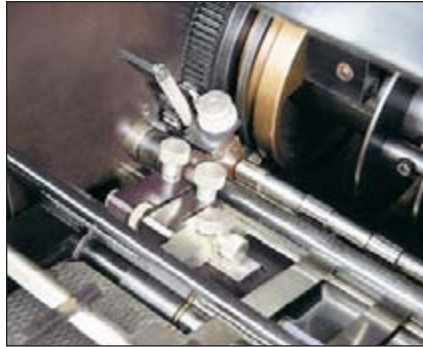
For multi-color work, the vacuum conveyor and pull guides ensure consistent, accurate register sheet after sheet.
