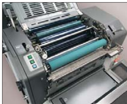
A uniform dampening supply to the plate surface enables sharper halftones, glossy solids and detailed fine text.
