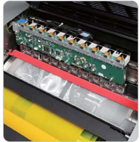
The Presstek 52DI incorporates 10 multi-beam laser diodes on each of its imaging modules.
