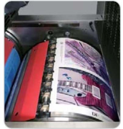
The sheet moves through the printing process on the 52DI's central impression cylinder without tail whip, resulting in first sheet registration.
