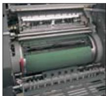
Plate clamps accept both pin bar and straight edge plates. Use metal or polyester material.
