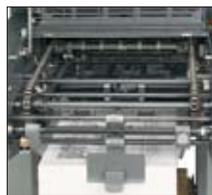
The chain delivery will neatly stack up to 20" of printed material and is easy to unload.
