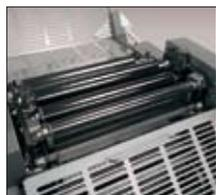
A bridge roller between the water and ink units makes roller cleaning quick and easy.
