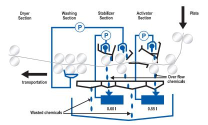
The SDP-Eco1630IIIR features a self-contained Eco processor that operates with two, ready-touse solutions for processing Silver DigiPlate. This unique processing technology uses 2/3 less Activator and Stabilizer than other systems.
