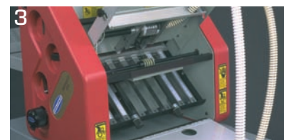
EASY ACCESS A swing-away feed table allows easy access to the lower fold plate.
