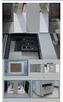
Ultrasonic double detect with sheet eject
