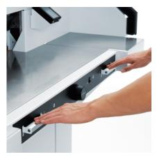
EASY CUT BLADE ACTIVATION BARS Patented EASY CUT blade activation bars ensure true, two-hand operation and allow blade and clamp to be activated independently.
